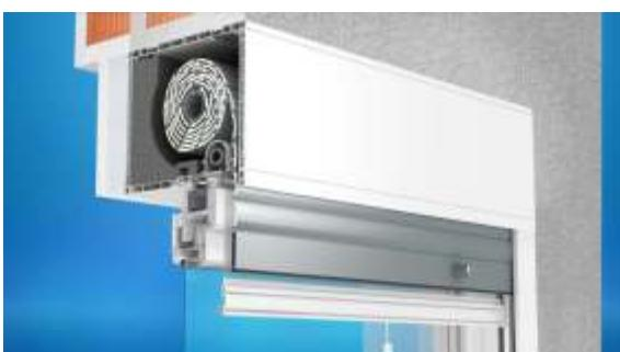
The TP1000K roller shutter is installed from the internal side. The internal front profile is grooved and equipped with a plaster slat. In order to have a more aesthetic look, the external front profile is smooth. The revision hatch in this type of system occurs from the bottom and the roller shutter is operated from the inside.
