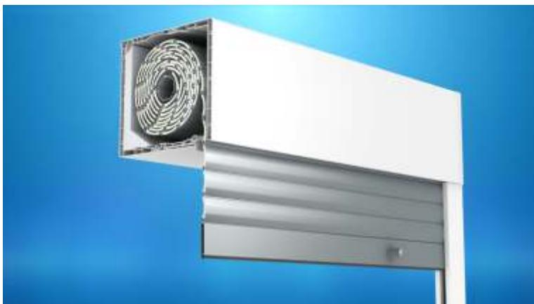
CC1000 is a basic system of top mounted roller shutters. The inspection hatch is mounted on the front part of the shutter box. They can be installed on windows which frame's max. thickness does not exceed 95 mm. This system cannot have mosquito net. CC1000 roller shutters system is perfect solution for houses and industrial facilities.
