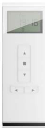
PX-15T - 15-channel remote control with Timer
