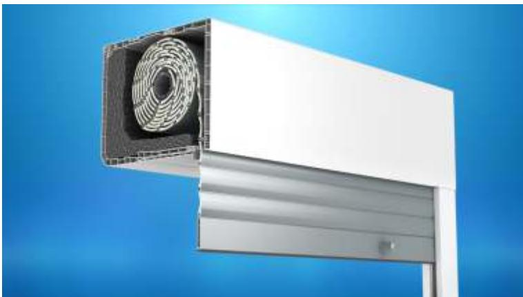
MX1200 is a system of roller shutters dedicated for renovation and monoblock windows. The specific construction of the shutter box with an inspection hatch at the front allows for mounting a roller shutter on the window frames of 60 to 180mm. The rounded bottom edge of the inspection hatch and the ability to use end caps on the access cover and the box sides increase the aesthetics significantly. The operation is possible both manual using a tape and electric using a switch or a remote control.
