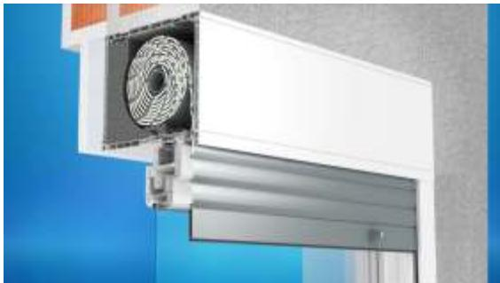
The TP1000K roller shutter is installed from the internal side. The internal front profile is grooved and equipped with a plaster slat. In order to have a more aesthetic look, the external front profile is smooth.
