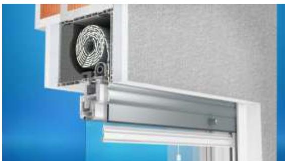
The TP1000K roller shutter is installed from the internal and external side. Front profiles additionally rifled and additionally equipped with plaster slats facilitate the installation. The revision hatch in this type of system occurs from the bottom and the roller shutter is operated from the inside.
